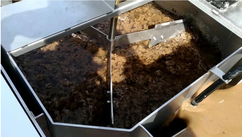
Fig. 13: Polymer effect – optimal flocks
