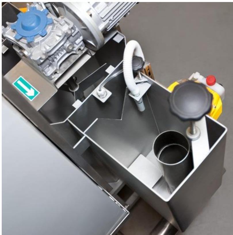
Fig. 7 – Setting the water level in the inlet chamber
