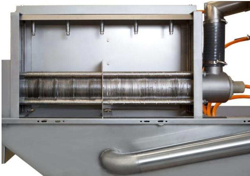
Fig. 14: Screw and washing system
